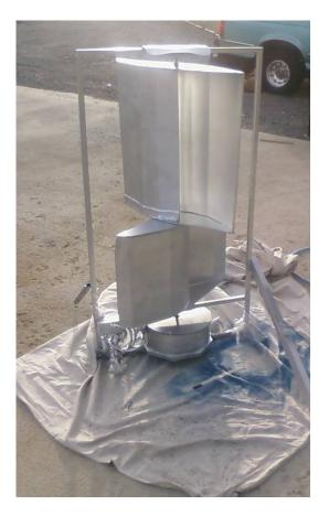
Completed 165 watt @ 28 MPH winds designed and build by Joseph Ellsworth Winter 2008. Includes PMG alternator capable of reaching 48 V charging aat 80 RPM or 12 MPH winds.
